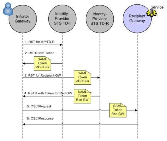
Figure 5: Role-based federation in the push-model
