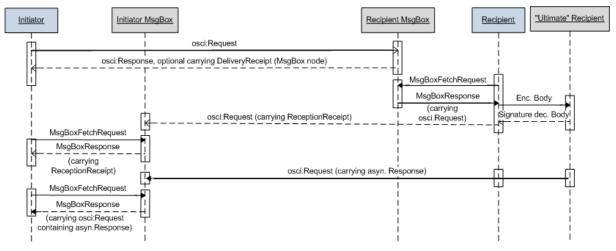
Figure 4: Sequence: MEP Initiator sends request to Recipients MsgBox
