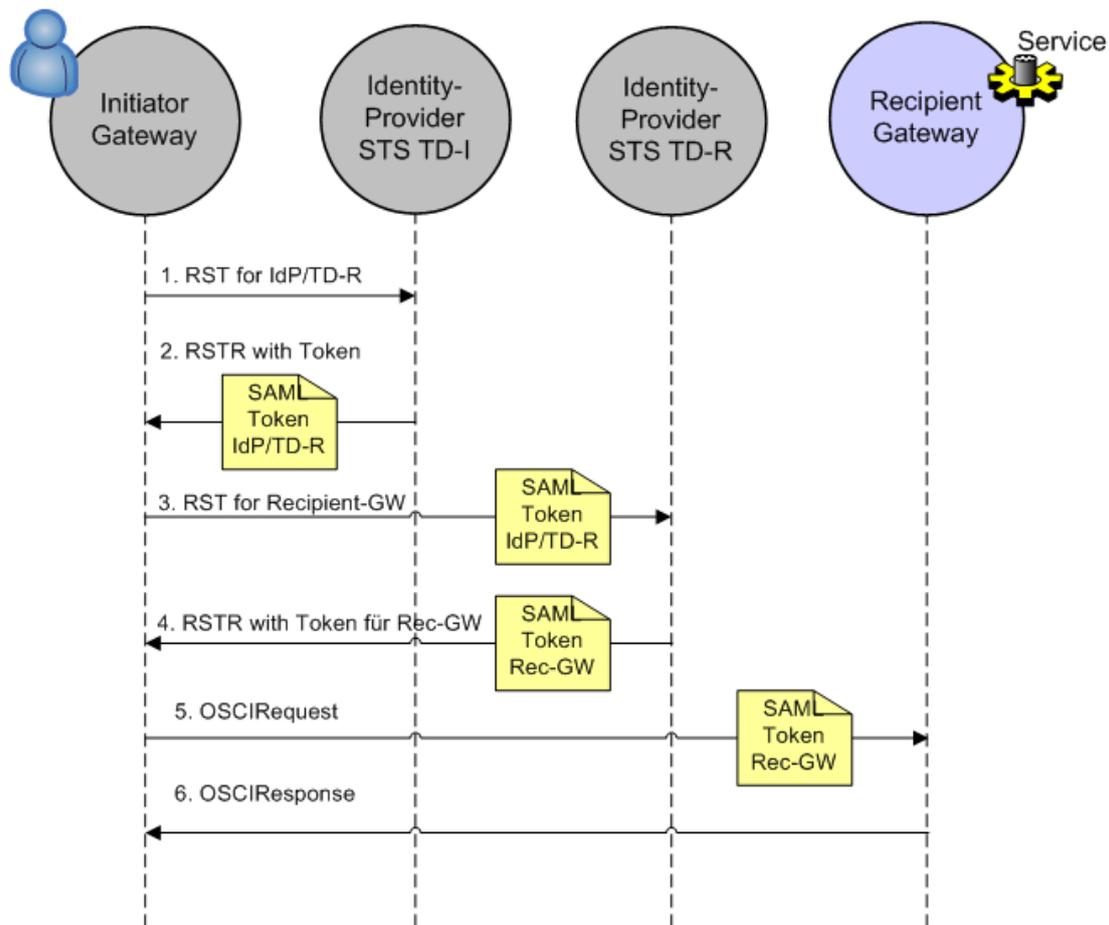
Figure 5: Role-based federation in the push-model
